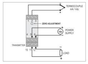
Figure 13 - TxlsoRail 0-10 Vdc - Thermocouple, mA, Vdc
