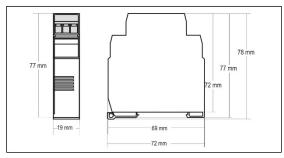
Figure 9 - Transmitter dimensions
