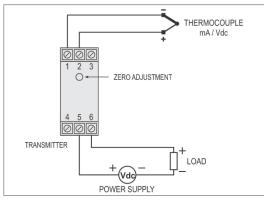
Figure 11 - TxlsoRail 4-20 mA - Thermocouple, mA, Vdc
