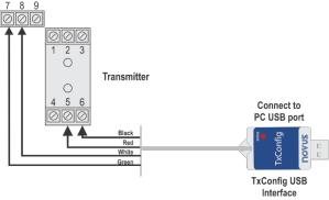
Figure 1 – TxConfig Interface USB connections
