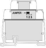
Figure 14 – Jumper position for 0-10 Vdc input
