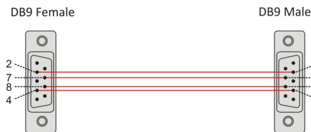
Fig. 26 – Building an extension cable
